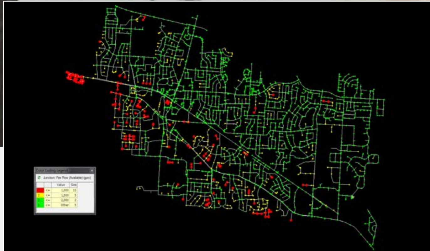
Navigate the network and map elements that satisfy (or not) fire flow constraints using WaterGEMS.
