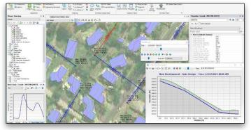
Terrain models can dynamically update node ground elevations, display surface contours and profiles, and design conduit inverts using real topography.
