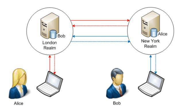
For more than two realms to trust each other, additional trust relationships must be established. Trusted realms cannot inherit or transfer trust from other realms. Trusted realm authentication only occurs between realms that have a direct, explicit trust relationship. In the previous example, even if the London realm were to add Paris as a trusted realm, New York and Paris would not trust each other unless you created a trust relationship between New York and Paris.
