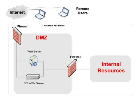
The following figure shows a basic network configuration after Authentication Manager integration.
