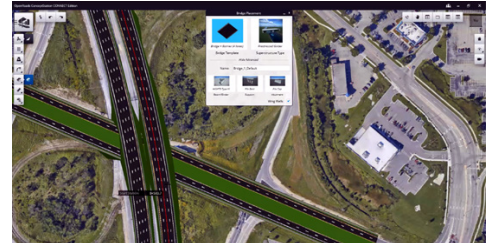
Road design leveraging a reality mesh in Bentley's OpenRoads™ ConceptStation.
